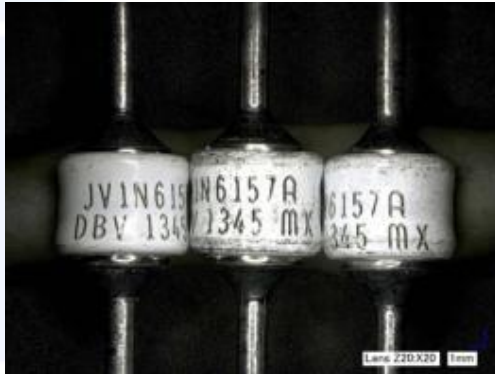
External Visual Inspection
